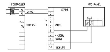
The SIA08 can be customized to accept custom (±15VDC) input signals and output a standard output signals. Other custom input and output configurations are available upon request.
