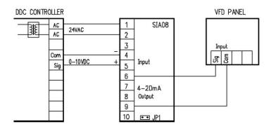
The SIA08 was designed to provide signal isolation for interfacing between DDC analog control systems to variable frequency drives. The SIA08 uses an on-board isolation transformer and linear optical coupler to provide input to output signal and power supply. The SIA08's input is on terminal 4 & 5, with JP1-4 jumper to select between: 0-10VDC, 0-5VDC, 0-1VDC, and 4-20mA. The SIA08 4-20mA output is found between terminals 6 and 9 (com).
