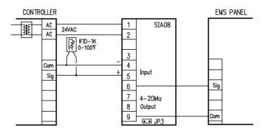
The SIA08 can be customized for a custom voltage or current input signals. The SIA08s input can be customized to have a high input impedance so that it will not cause any loading of the original circuit. The sensor signal is isolated from the output and scaled to the desired voltage or current range.
