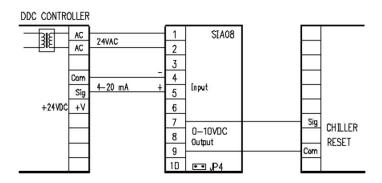
The SIA08 was designed to provide signal isolation for interfacing between VFDs, chillers, humidifiers, EMS systems, valves, etc. to DDC analog control systems. The SIA08 uses an on-board isolation transformer to avoid ground loops due to half and full-wave power supply sections powered from a grounded 24VAC source and other ground loop potentials.
