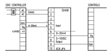
The SIA08 can be customized for a custom voltage or current output signals from a standard input signal. Other custom input and output configurations are available upon request.
