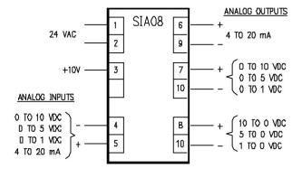
NOTE: MULTIPLE INPUTS AND OUTPUTS ARE SHOWN BUT ARE NOT SIMULTANEOUS
